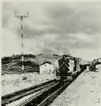
All switches and signal lights on Orinoco Mining Company's ore railroad are radio-activated.
